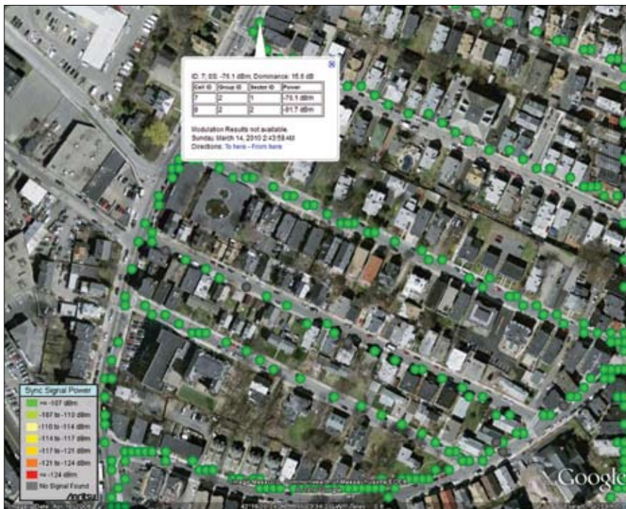
Figure 5: LTE coverage map opened in Google Earth
